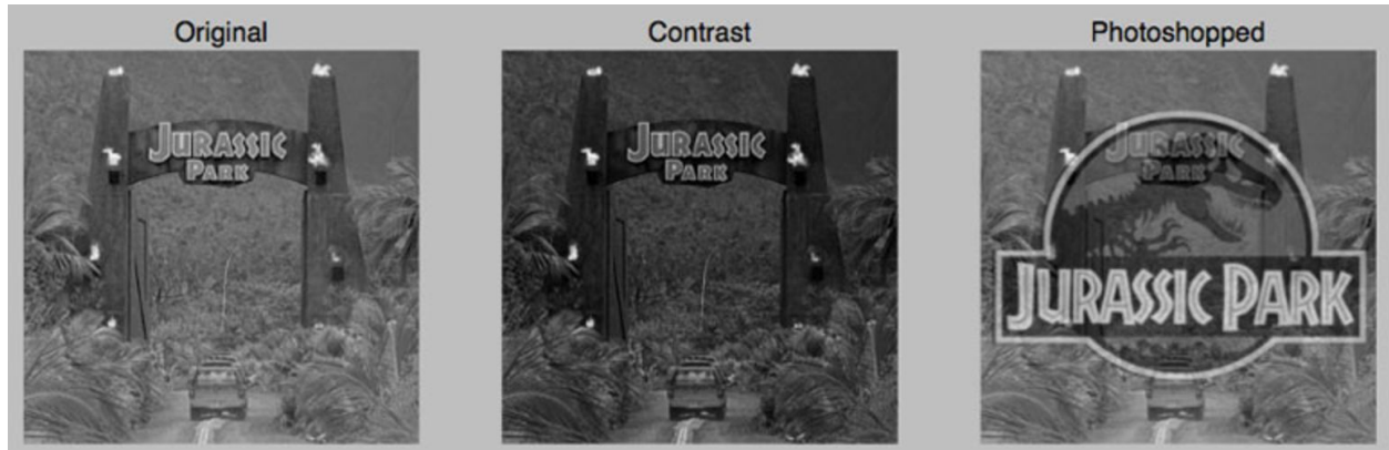
Figure C1 - A comparison between the MSE and SSIM methods for evaluating similarity between images (taken from [5]). Contrast: MSE=1401, SSIM=0.78 and Photoshopped: MSE=1077, SSIM=0.69
